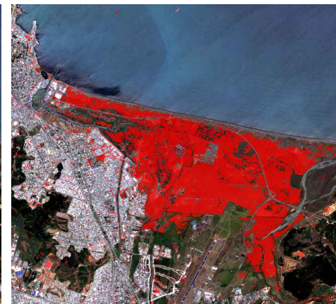
Image: RapidEye image of Concepción on February 27, 2010. The red marked areas show the damaged areas after the quake hit the city.
