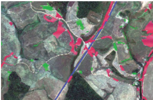
Pipeline Monitoring: The image illustrates changes along a pipeline (blue line). Critical changes like vegetation encroachment or construction activities are visualized in red, all other changes are shown in green.
